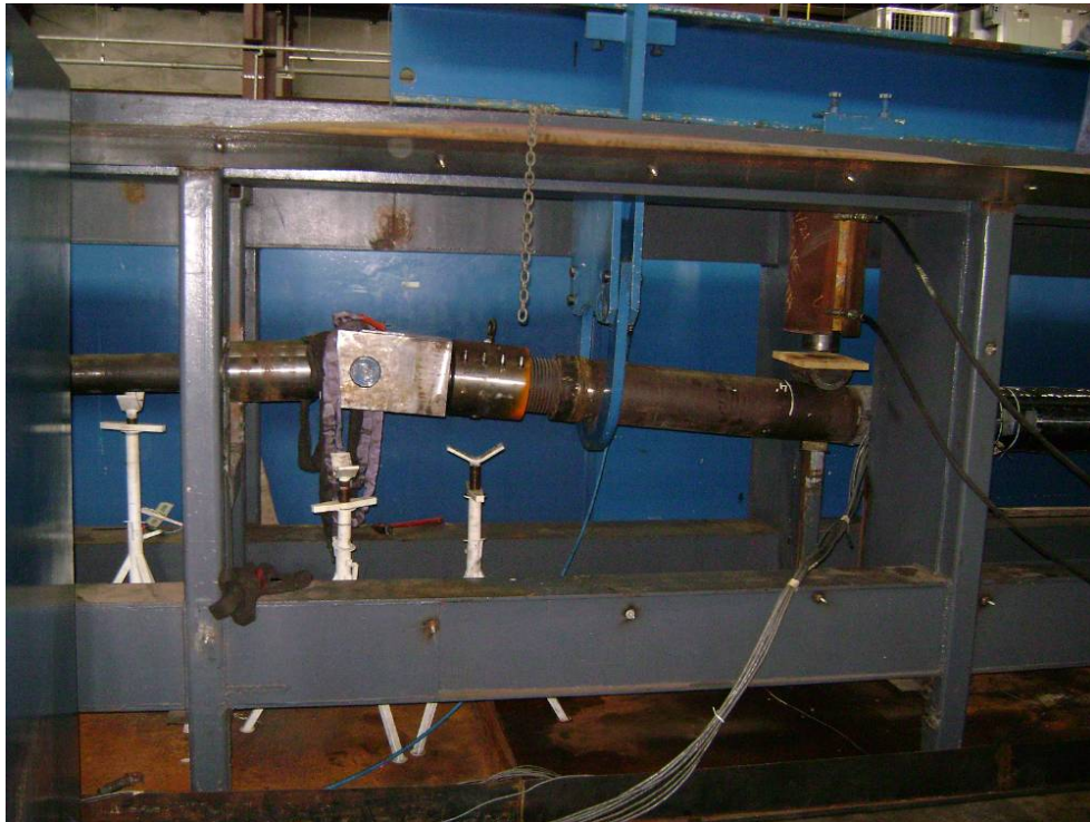
Figure 72 – Photograph showing displaced configuration of bending sample
