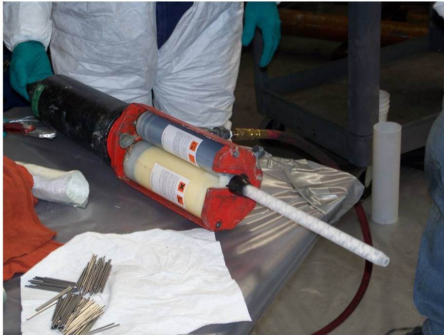
Figure 50 – Epoxy mixing gun used to mix the epoxy Spabond 340 adhesive
