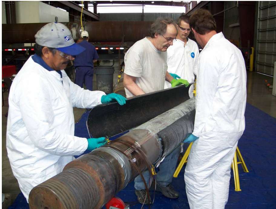
Figure 52 – Installation of the carbon half shells
