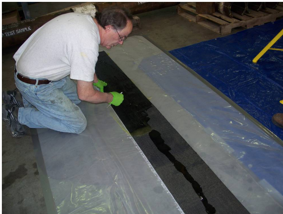
Figure 47 – Saturating the uniaxial stitched carbon cloth
