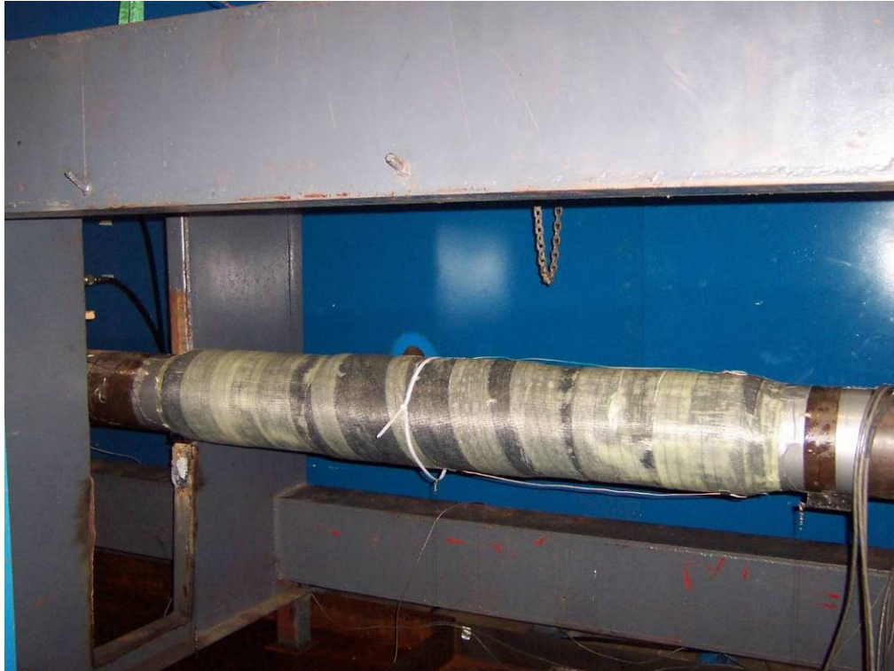
Figure 16 – Photo showing Product C prior to bend testing
