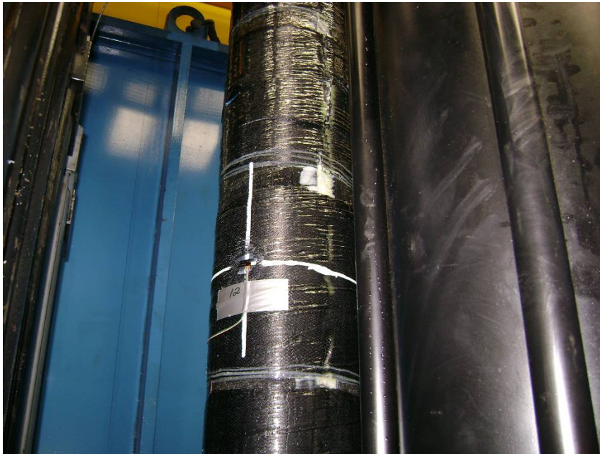
Figure 70 – Photo of tension test showing fracture
