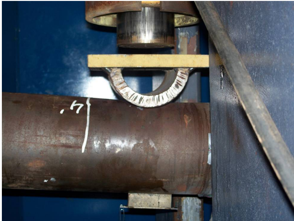
Figure 65 – Plastic deformation near the hydraulic cylinder point of contact
