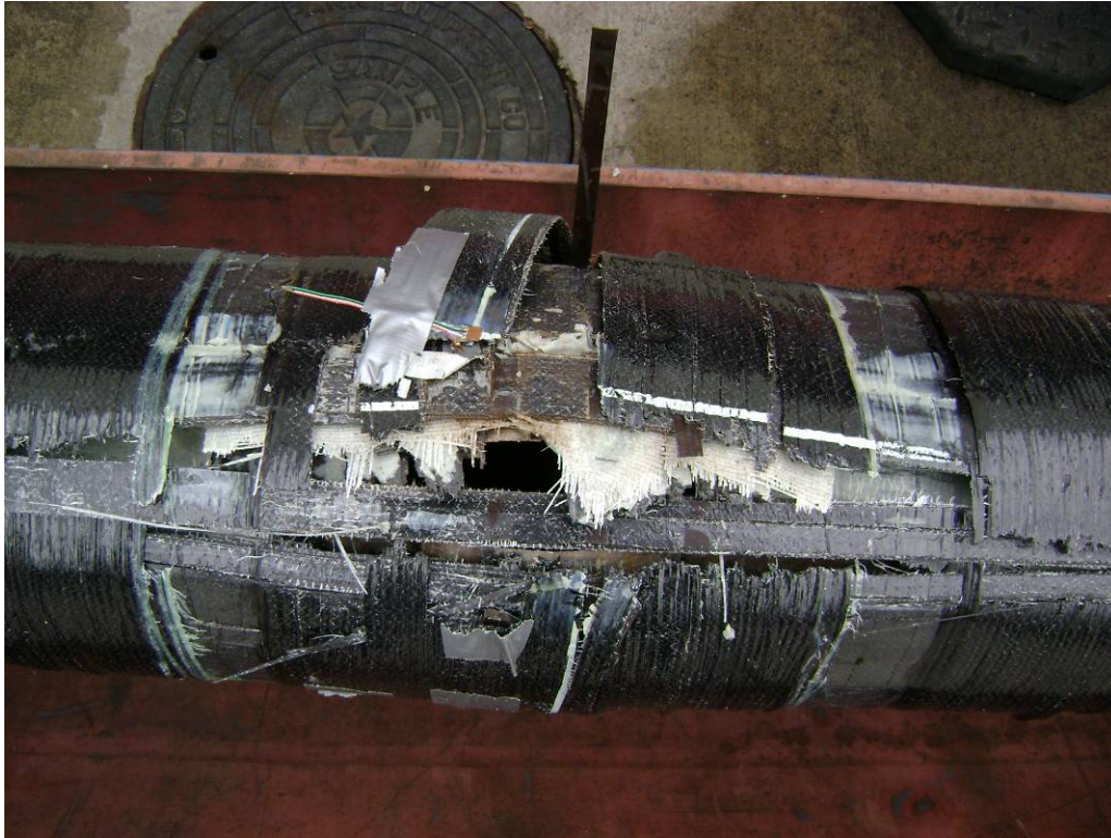
Figure 68 – Photo of burst test sample showing failure
