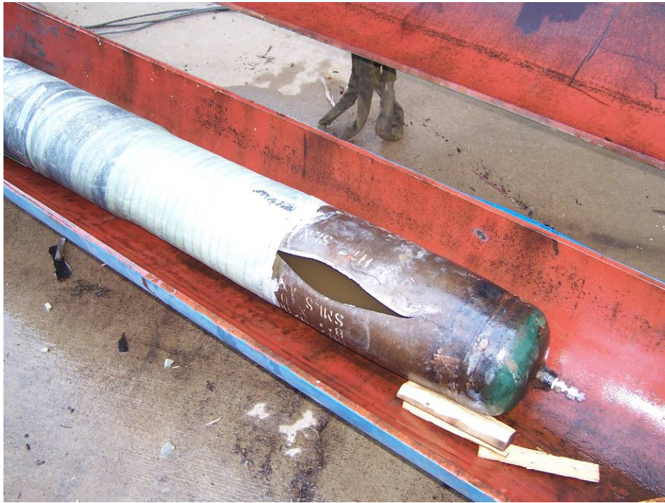
Figure 12 – Failure in burst sample using Product C
